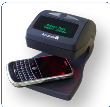
The BGR120S reading a bar code from the screen of a PDA
