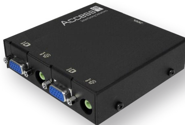
EXT200 receiver showing two audio and video output connectors
