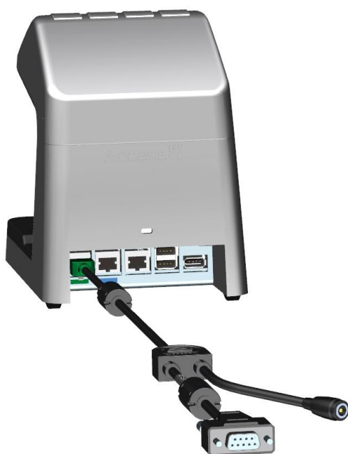
Figure 2: Serial connection cable
