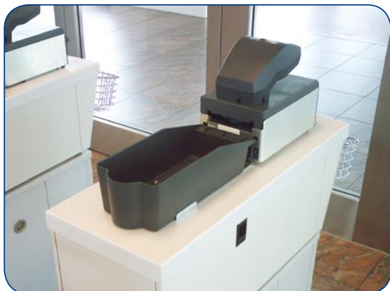
Access BGR adaptor on an IER627 document bin, concealing cables
