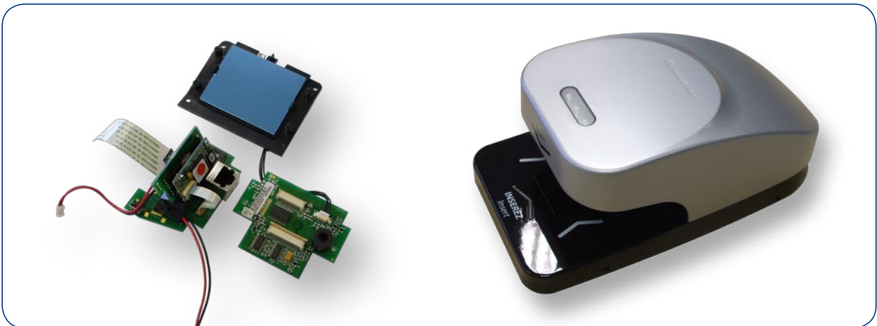
The 2D bar code reading kit from Access and the finished product manufactured by Fortress GB, the combined bar coded and RFID ticket reader.
