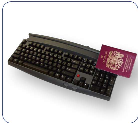
The Access ATB integrated keyboard reading a passport
